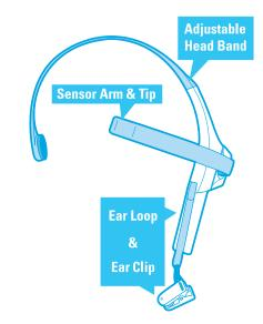
How to Wear the MindWave Headset Should rest on the head as shown with the sensor tip touching the forehead, the ear loop behind the ear and the clip attached.
