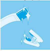
• For travel and storage, gently push the sensor arm up until it is aligned with the top of the headset. Be careful not to overextend the maximum range of the boom by adjusting it beyond the natural stopping point.
